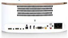
The Philips Screeneo U3 has a comprehensive array of connections (HDMI, VGA, audio and headphone port, USB, etc.) enabling it to be
