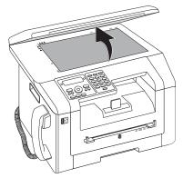
2 Lay the document onto the scanner glass with the written side down.
