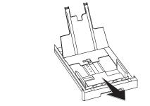
3 Adjust the length of the paper tray to the printer paper. Press the lock key on the base of the paper tray. Slide the rear panel until it snaps into the suitable marking: Legal = LG, A4 = A4, A5 = A5, Letter = LE, B5 = B5.
