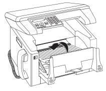
7 Place the toner cartridge into your device. The cartridge should snap securely into position.
