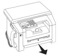
**3** Push the paper tray into the device all the way to the stopping point.
