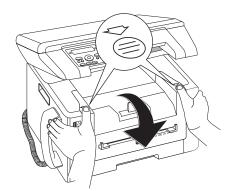
3 Remove the toner cartridge by gripping the handle in the middle and pulling it forwards out of the device
