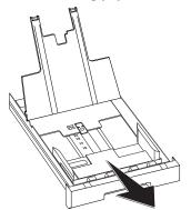
4 Removing the tape in the paper tray which was used for transportation purposes.
