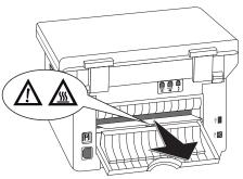
4 Close the paper jam flap. The fuser levers will automatically fold into starting position when the paper jam cover is closed.
