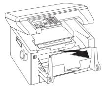
4 Remove the tape and protective paper, but do not remove the protective strip from the car-tridge yet.
