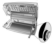
5 Close the device. Insert the paper tray in the opening provided for it behind the paper feeder. Insert paper again.
