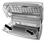
9 Break the chip card from the Plug'n'Print card. Insert the chip card in the plug socket on the left hand side next to the ink film tray.
