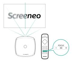
Auto focus adjustment is also available. You can enable or disable auto focus adjustment. Press **OPTION** and go to *Image – Autofocus Settings.* If enabled, the projector will re-focus automatically when you reposition the projector.
