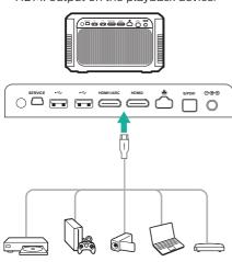
2 Press SOURCE 1 to access and select HDMI 1 or HDMI 2 input source.
