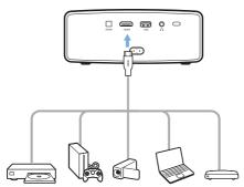
2 The projector automatically switches to HDMI input when HDMI connection is made. The projection screen shows images. If the projection screen does not show images, select HDMI input manually. Press (○■)/◆□ to access the settings options and go to Input Source - HDMI.
