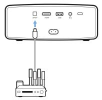
2 To output audio to the external device, make sure external speaker output is activated. Press (○■)/←1 to access the settings options and go to Audio Output - ARC/Optical.
