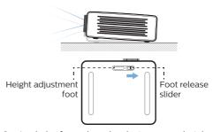
2 Lock the foot when the desire screen height is reached. Simply release the slider to lock the foot.
