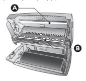
Clean the feed roller (A) and the underside of the support pad of the feeder roller (B) with a soft, lintfree cloth moistened with cleaning alcohol (96 percent). Rotate the feed roller; You must clean the entire roller.
