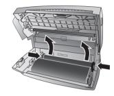
Remove both the rolls from the device. The used ink film cannot be reused.
