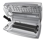
Place the smaller roll without ink film in the front tray. The blue gear wheel must be on the right hand side and the pin must be inserted in the depression on the left hand side.
