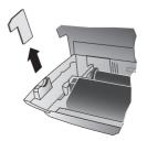
Carefully remove the rubber bands from the new ink film. Make sure that the film is not damaged!
