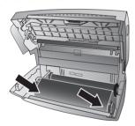
Break the chip card from the Plug'n'Print card. Insert the chip card in the plug socket on the left hand side next to the ink film tray.
