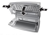
Carefully pull the document to the front or to the back out of the device.
