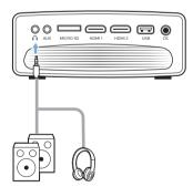
When connecting to the headphones, use the volume control on the remote control to adjust the volume to a comfortable level.
