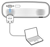
On your computer, adjust the screen resolution of the computer to the correct setting and switch the VGA signal to an external monitor. The following resolutions are supported:
