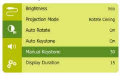
2 Press the Navigation button to adjust the image shape.
