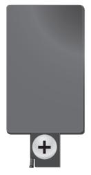
**3** Push the battery compartment back into the remote control until the locking mechanism engages.
