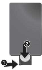
2 Insert the new batteries into the battery compartment with the positive and negative poles as shown on the back of the remote control. Make sure the polarities(+ and -) are aligned correctly.
