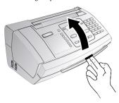
Lock the cover of the device completely into place when opening the device. You could be injured if the cover falls while you are working on the device.
