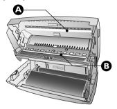
**5** Clean the feed roller (**A**) and the underside of the support pad of the feeder roller (B) with a soft, lint-free cloth moistened with cleaning alcohol (96 percent). Rotate the feed roller: You must clean the entire roller.
