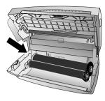
8 Place the smaller roll without ink film in the front tray. The blue gear wheel must be on the right hand side and the pin must be inserted in the depression on the left hand side.
