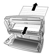
5 Close the scanner cover and the cover of the automatic document feeder. Both the supports must securely snap into place. **6** Turn the blue gear wheel forward to tension the ink film. The ink film must not have any creases.
