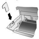
**10** Turn the blue gear wheel forward to tension the ink film. The ink film must not have any creases.
