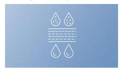
A 4 stage filtration system filters out a wide range of pollutants for superior, long-lasting performance. The CP filter reduces large particles and absorbs chlorine, pesticides and chemicals. Then the RO filter removes total dissolved solids in the water. Finally, the water goes through the mineraliser filter to be enhanced with minerals and further improve the taste.
