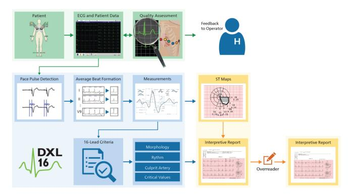
From acquisition to report generation, the Philips DXL 16-Lead Algorithm uses multiple steps to ensure a high quality interpretation.
