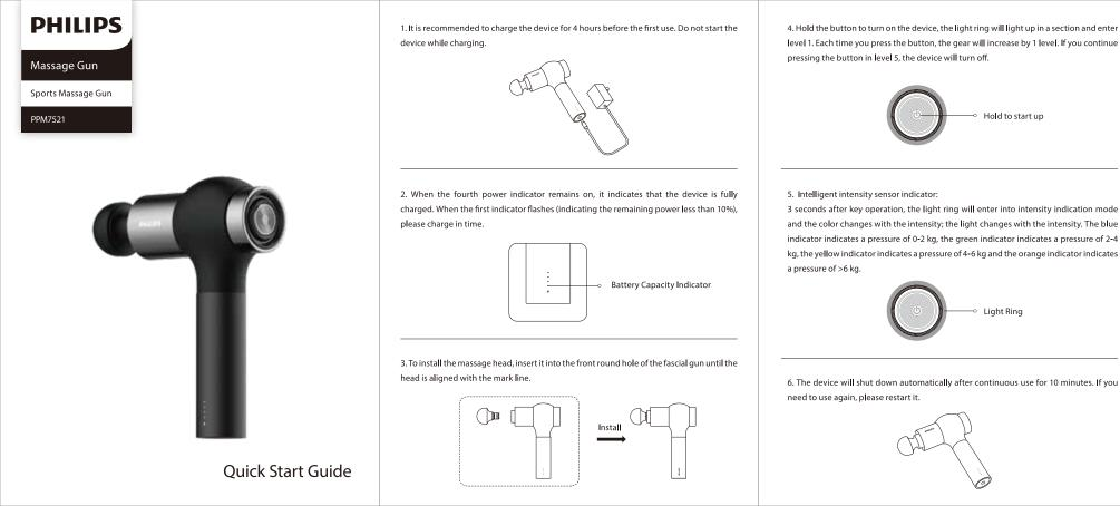
3 seconds after key operation, the light ring will enter into intensity indication mode and the color changes with the intensity; the light changes with the intensity. The blue indicator indicates a pressure of 0-2 kg, the green indicator indicates a pressure of 2-4 kg, the yellow indicator indicates a pressure of 4-6 kg and the orange indicator indicates Light Ring
