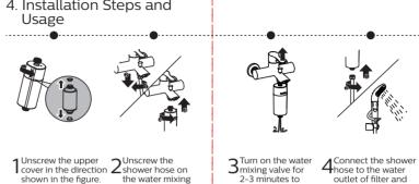
Please use the municipal tap water as the nlet water. (Please do not use water of any unknown source): Do not install it if the water supply pipeline is with a water pressure exceeding 0.4 MPa. If the pressure exceeds 0.4 MPa, the pressure reducing valve shall be added (to be purchased The inlet water temperature of this shower filter should be 5 - 60°C as required. If hot water over 60°C has been used for a long time, the filter may be damaged. When the indoor tighten them, then
