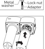
3) Installation of the filter cartridge • Screw the cartridge into the filter cover according to their respective positions and the direction shown in the figure.
