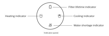
When the dispenser is heating up the water in the hot water tank, the heating indicator light will be on.
