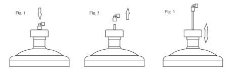
Note: If there is not a secure connection between the hose cap and the connector on the water dispenser, the water pump will operate but the water dispenser will not dispense water. Make sure the hose is connected to the water dispenser correctly.
