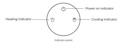
When the dispenser is connected with power and the power button switches to ON, the power on indicator will light up.
