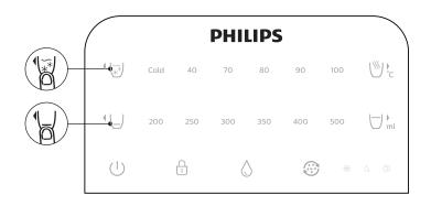
• Long press both buttons 🗑 🖵 for 3 seconds to reset the filter lifetime.
