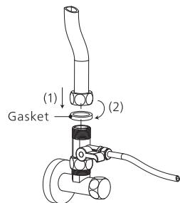
e. Switch off the three-way ball valve.
