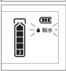
(3) Water production icon: When the water filtration system is working, the "Water Production" icon will flash.
