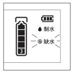
(4) When the water flow is too low, which means probably the filter needs to be replaced, the "Water Shortage" icon will flash.
