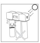
① Do not install in direct sunlight or any place where it may be exposed to hazardous chemicals, or where it may be damaged, such as falling, being hit, etc..
