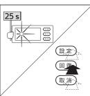
(2) When the screen is not displayed, push any key to light up the display screen for 25 seconds.
