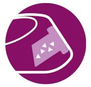
Our specially designed and built-in calc container collects calc particles during ironing. The Self Clean process flushes the calc out of the iron to maintain consistent ironing performance day after day.
