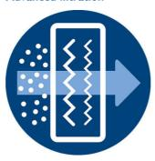
A multi-layer filtration system filters out a wide range of pollutants for superior, long-lasting performance. The pre-filter removes larger dust and hair. Then the true HEPA filter removes ultrafine particles. Finally, an active carbon filter absorbs harmful gases.
