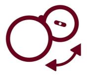
The filter holder is opened by swinging it to the side, which makes the filling of coffee easy. The filter holder is also detachable, for easy cleaning.
