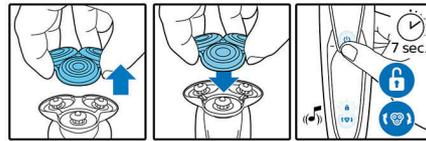
1. Pull the shaving head holder off. 2. Replace the shavings heads with new ones. 3. Reattach the shaving head holder. 4. To reset the shaver, press and hold the on/off button for more than 5 seconds.
