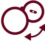
The filter holder is opened by swinging it to the side,
