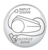
This powerful 2000 Watt motor generates max. 400 Watt suction power for excellent cleaning results.
