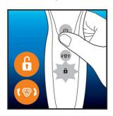
After replacing shaving heads, you can reset the replacement reminder by pressing the on/off button for more than 7 seconds. Otherwise, replacement trigger will turn off automatically after 9 successive shaves.
