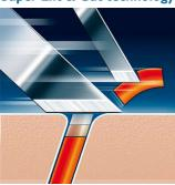
Dual blade system of your Philips shaver: first blade lifts, second blade cuts for a comfortable close shave.
