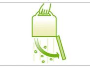
The closed dust container of the Philips bagless vacuum cleaner can be emptied by the bottom by the simple push of a button.
