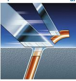
The dual blade system of this electric shaver lifts hairs to cut comfortably below skin level.
