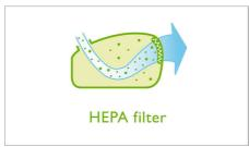
This HEPA filter catches harmful microscopic vermin that causes respiratory allergies. To maintain effective fitration, replace the HEPA filter every 6 months.
