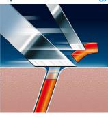
The dual blade system of this electric shaver lifts hairs to cut comfortably below skin level.
