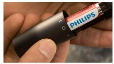
To change the battery, rotate the handle and open the device to reach the battery compartment.
