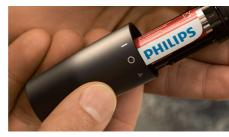
To change the battery, rotate the handle and open the device to reach the battery compartment.
