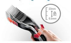
Designed for a hassle-free cutting experience and easier storage, one adjustable comb offers every length setting you will need. Simply adjust the comb to select and lock in the length you want, with 23 length settings from 1 to 23mm (3/64" to 7/8"), and precisely 1mm (3/64") between each length. Or you can use it without the comb for a close 0.5mm (1/32") trim.
