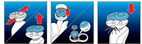
1. Press the release buttons on the shaving unit and pull the shaving head holder off the shaving unit.
