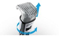
Zoom wheel makes it easy to adjust the comb in the 12 length settings. The settings offer ultimate precision of 0.5mm steps on the shorter lengths to define exactly the style you want, between a 5 o'clock shade and 3 days stubble. Also for the longer beards it offer exactly the lengths you need in 1 mm step sizes.
