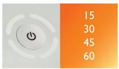
Set the timer according to your needs to 15, 30, 45, 60 minutes and choose the right brightness out of the three levels by using the dimmer.
