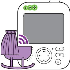
Note: The link light shows that the parent unit is still on and connected to the baby unit.
