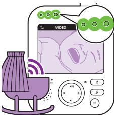
When the baby unit picks up a sound, one or more sound level lights on the parent unit light up green. The number of lights that go on depends on the loudness of the sound picked up by the baby unit. The louder your baby cries, more sound level lights light up green.
