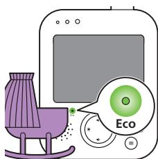
When the ECO mode is activated the display and sound of the parent unit switch off when no sound is detected for 20 seconds. The ECO light lights up green to indicate that the ECO mode is activated. During ECO mode the display and sound transmissions are turned off.
