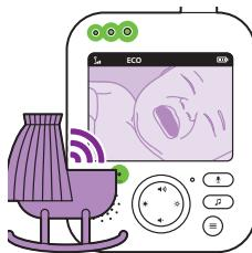
When sound is picked up by the baby unit, the display and sound of the parent unit switch on immediately. The sounds are transmitted to the parent unit and the sound level lights light up green. As long as no sound is detected, the sound level lights are off.
