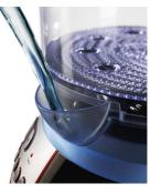
External water inlet for refilling reservoir during use.
