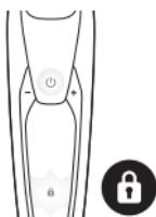
While you activate the travel lock, the travel lock symbol lights up white continuously. When the travel lock is activated, the appliance produces a sound and the travel lock symbol flashes.
