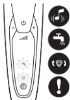
If the shaving heads are blocked, the exclamation mark lights up orange continuously. The replacement reminder and the cleaning reminder flash white alternately and you hear a sound. In this case, the motor cannot run because the shaving heads are soiled or damaged.
