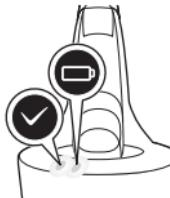
When the cleaning program is done, the ready symbol lights up continuously.
