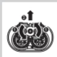
**3** To remove the retaining frame, turn the central spring clockwise (1). Then lift the retaining frame out of the shaving unit (2).
