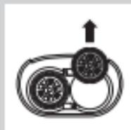
**4** Lift the shaving heads out of the shaving unit. Remove and clean one shaving head at a time. Each shaving head consists of a cutter and a guard.
