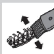
**6** Clean the cutter with the cleaning brush. Brush carefully in the direction of the arrows.
