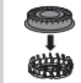
**8** Put the cutter back into the guard after cleaning.
