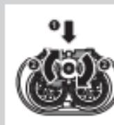
**10** Put the retaining frame back into the shaving unit (1), and turn the central spring anti clockwise (2).
