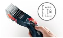
Simply select and lock in the length you want with the adjustable comb which provides 12 lock-in length settings from 1mm to 23mm, with precisely 2mm between each length. Or you can use it without the comb for a close 0.5mm trim.
