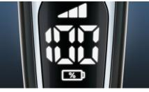
The intuitive display shows relevant information, enabling you to get the best performance out of your shaver: - 3 digit (%) battery indicator - Cleaning Indicator - Battery Low Indicator - Replacement Head Indicator -Travel Lock Indicator
