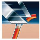
Dual blade system of your Philips shaver: first blade lifts, second blade cuts for a comfortable close shave. HQ9/32
