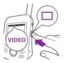
Press the mode button on the side of the parent unit to select the VIDEO mode.
