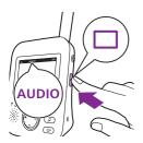
**1** Press the mode button on the side of the parent unit to switch to AUDIO mode.
