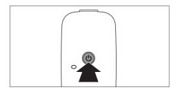
Press and hold the **૭** button on the parent unit for 3 seconds until the 'link' light starts flashing red.
