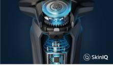
The electric shaver has an intelligent facialhair sensor that reads hair density 125 times per second. The technology auto-adapts cutting power for an effortless and gentle shave.
