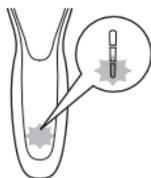
When the battery is almost empty, the bottom light of the battery charge indicator flashes orange.
