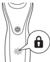
While you activate the travel lock, the travel lock symbol lights up continuously. When the travel lock is activated, the travel lock symbol flashes.
