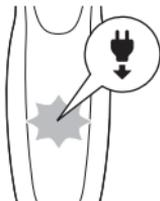
The 'unplug for use' symbol flashes to remind you that you have to disconnect the appliance from the wall socket before you can switch it on.
