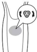
For maximum shaving performance, we advise you to replace the shaving heads every two years. The appliance is equipped with a replacement reminder which reminds you to replace the shaving heads. The shaving unit symbol lights up and the arrows flash to indicate that you have to replace the shaving heads.
