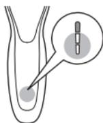
The remaining battery charge is shown by the lights of the battery charge indicator that light up continuously.
