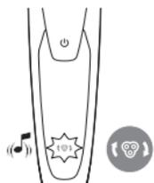
The replacement reminder indicates that the shaving heads need to be replaced. The shaving unit symbol lights up continuously, the arrows flash white and you hear a beep when you switch off the shaver.
