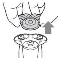
**3** Switch off the shaver. Pull the shaving head holder off the bottom part of the shaving unit.
