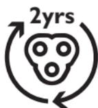
For maximum shaving performance, we advise you to replace the shaving heads every two years. Replace damaged shaving heads immediately. Always replace the shaving heads with original Philips shaving heads (see 'Ordering accessories'). Replacement reminder
