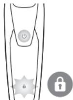
While you activate the travel lock, the travel lock symbol lights up white continuously. When the travel lock is activated, the appliance produces a sound and the travel lock symbol flashes.
